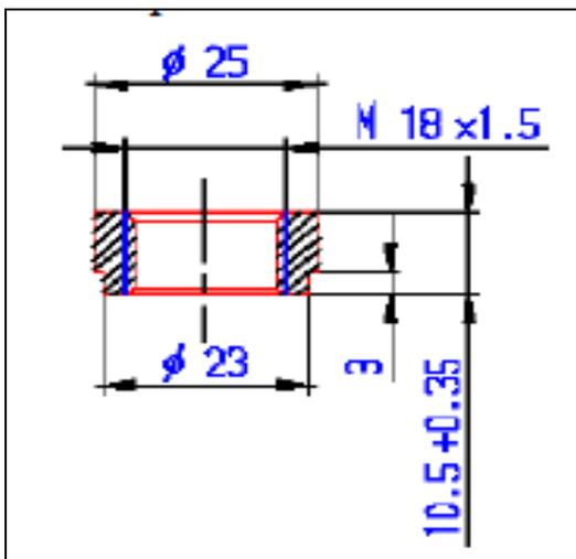
Figure 9- Sensor thread boss dimensions
