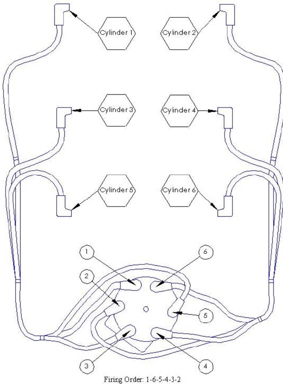
5.7L Engine Spark Plug Wire Routing Diagram
