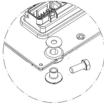
Figure 8- SECM mounting hardware
