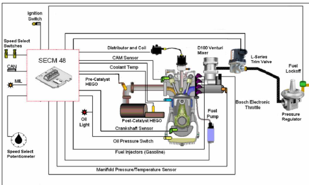
Figure 1- PG-08 Fuel System Engine in Certified Engines
