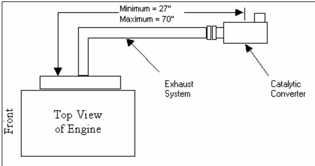
Figure 10- Catalytic converter mounting
